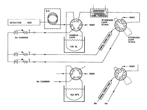
**Figure 1.** Configuration of the valving and cryotrap system for the analysis of organic mercury compounds using permeated DMHg calibration.
